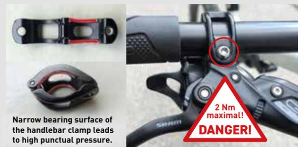
If this type of clamping design is used, do not exceed 2 Nm of torque when tightening the clamping screw. The handlebar can break otherwise if exposed to high pressure.
